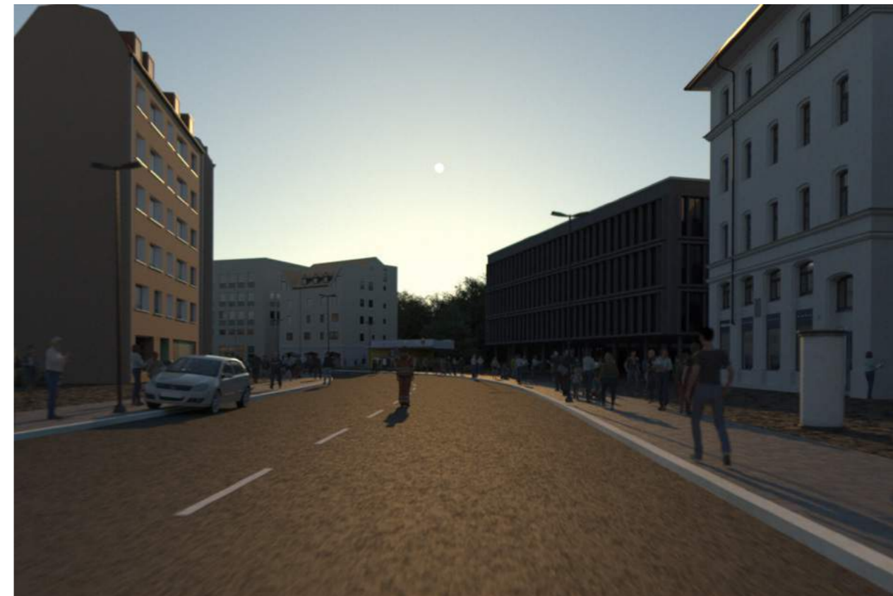
Raytracing generated synthetic image with procedural sun and physical sensor effects (© Robert Bosch GmbH | BIT Technology Solutions | Intel Corporation | Valeo Schalter und Sensoren GmbH)
