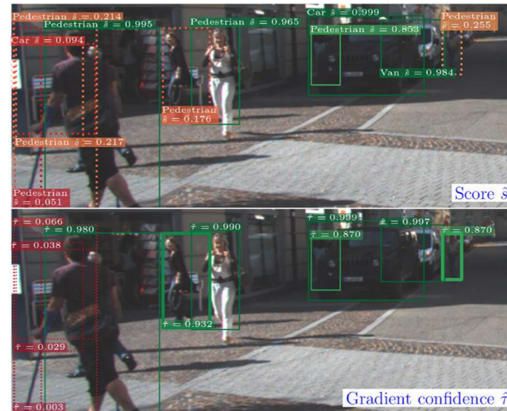
Comparison of network-intrinsic („Score“, top) and gradient-based confidence estimation (bottom) in a real-world street scene from the KITTI dataset (© BUW + KIT)
